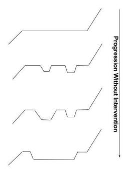
**Flat:** Does not drain effectively, progresses towards rutted, pot-holed and ultimately entrenched.
