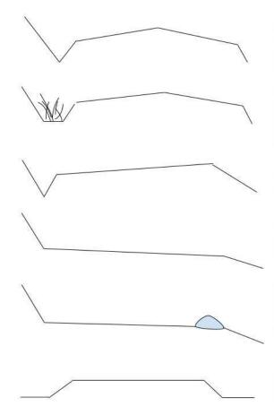
**Crowned:** 2-4% grade over the crown (less and drainage will be impeded and vehicles will cause ruts, more and vehicles will drive down the middle and cause ruts)
